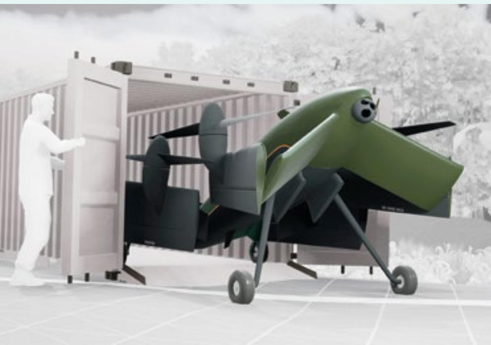
3 Pivots on back wheels to take off vertically
