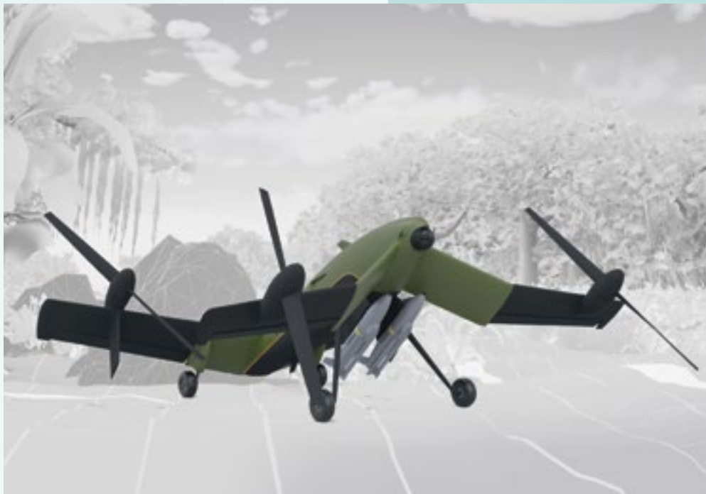
4 Leans forward to fly as a fixed-wing aircraft with long endurance
