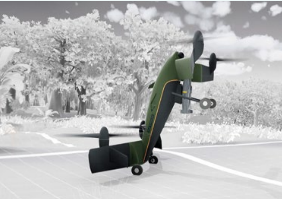
3 Pivots on back wheels to take off vertically
