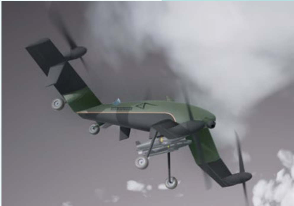
4 Leans forward to fly as a fixed-wing aircraft with long endurance
